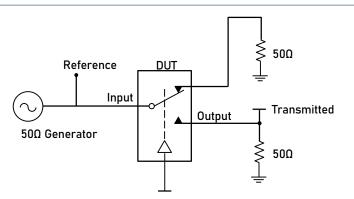
Channel switch control/s test socket is nomalized. Off isolation is measured across an off channel.On loss is the bandwidth of an On switch. $V_{\rm ISO}$ , Bandwidth and  $V_{\rm ONL}$  are independent of the input signal direction.
