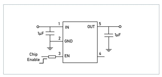
Note: The EN pin is not be suspended
