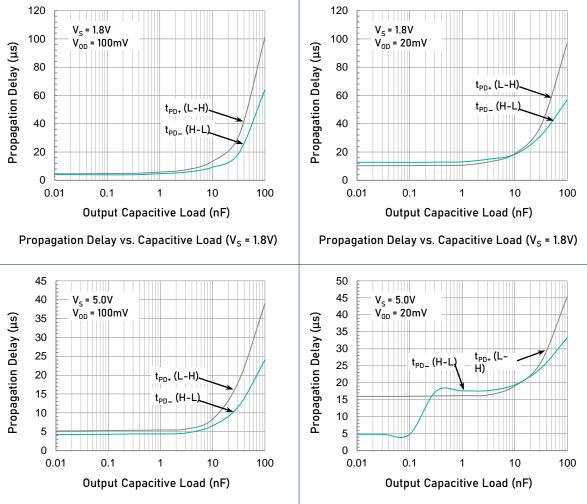
Propagation Delay vs. Capacitive Load (V<sub>s</sub> = 5.0V)
