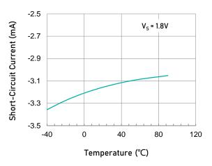
Short-Circuit Current vs. Temperature (V<sub>S</sub> = 1.8V)
