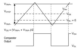
Figure 2. Input and Output Waveform, Non-inverting
