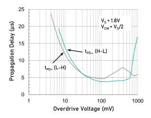
Propagation Delay vs. Input Overdrive  $(V_S = 1.8V)$
