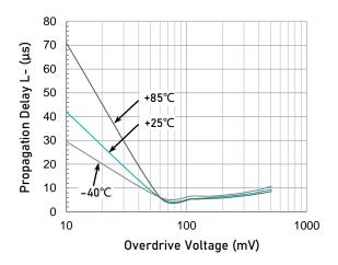
Propagation Delay H-L (tpp.) vs. Input Overdrive
