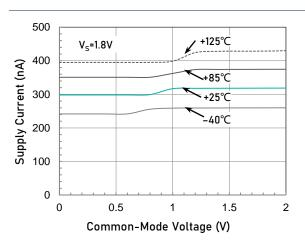
Supply Current vs. Common-Mode Input ( $V_S = 1.8V$ )
