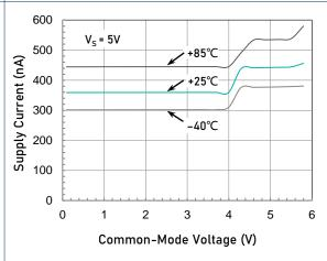
Supply Current vs. Common-Mode Input  $(V_S = 5.0V)$
