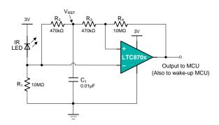
Figure 5. IR Receiver AFE Using LTC870x
