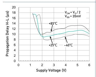
Propagation Delay H-L  $(t_{PD-})$  vs. Supply Voltage
