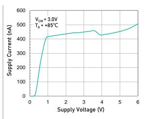
Supply Current vs. Supply Voltage
