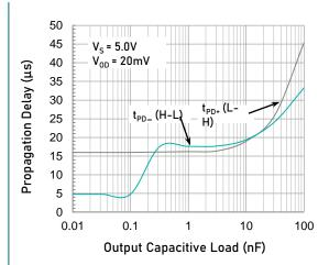
Propagation Delay vs. Capacitive Load ( $V_S = 5.0V$ )
