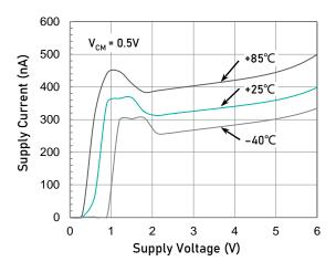
Supply Current vs. Supply Voltage
