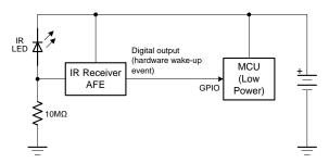
Figure 4. Coin Cell Battery Powered IR Receiver
