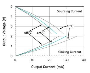
Output Voltage vs. Output Current
