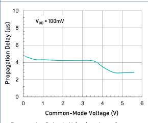
Propagation Delay L-H ( $t_{PD+}$ ) vs. Input Common-Mode Voltage
