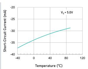
Short-Circuit Current vs. Temperature ( $V_S = 5.0V$ )
