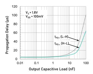
Propagation Delay vs. Capacitive Load ( $V_S = 1.8V$ )
