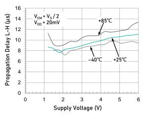
Propagation Delay L-H (t<sub>PD+</sub>) vs. Supply Voltage
