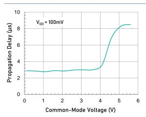
Propagation Delay H-L  $(t_{PD-})$  vs. Input Common-Mode Voltage
