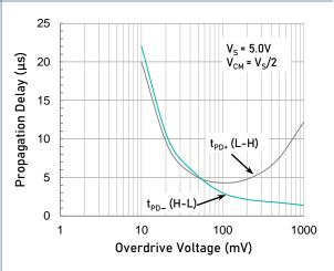
Propagation Delay vs. Input Overdrive ( $V_S = 5.0V$ )
