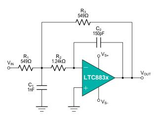
Figure 5. Second-Order, Butterworth, 500-kHz Low-Pass Filter
