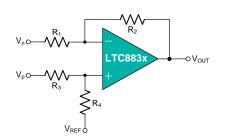
low-leakage cables that that is required to connect a pH probe (general purpose combination pH probes, e.g Corning 476540) to metering ICs such as ADC, AFE and/or MCU. A LTC883x op-amp and a lithium battery are housed in the probe assembly. A conventional low-cost coaxial cable can be used to carry the op-amp's output signal to subsequent ICs for pH reading.
