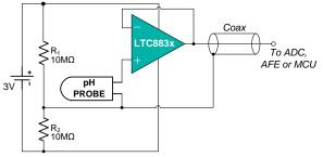
All components contained within the pH probe
