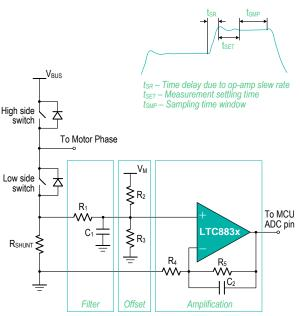
Figure 7. Current Shunt Monitor Circuit
