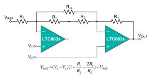
Figure 9. Instrumentation Amplifier
