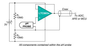
Figure 10. Buffered pH Probe
