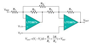
Figure 9. Instrumentation Amplifier
