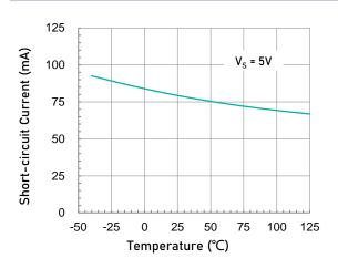
Short-circuit Current as a function of Temperature.
