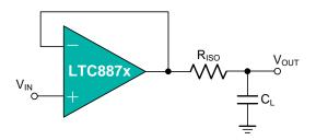
Figure 2. Indirectly Driving Heavy Capacitive Load
