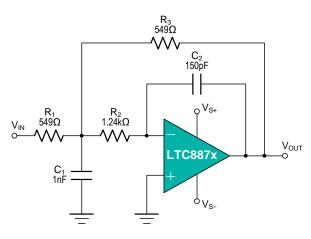
Figure 5. Second-Order, Butterworth, 500-kHz Low-Pass Filter
