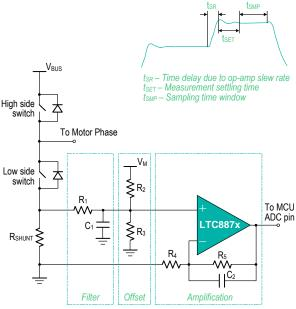
Figure 7. Current Shunt Monitor Circuit
